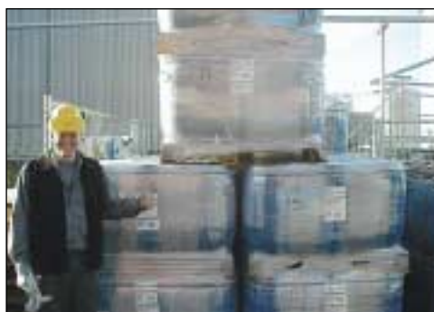
On arrival, the spent catalyst is tagged with a batch number and registered in the system that will track it all the way. Note how well packed the arriving catalyst is – a big help to speed things up, and safer to handle.
