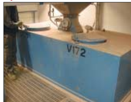
Dust and broken pieces are collected in another vessel, weighed 500 kg at a time...
