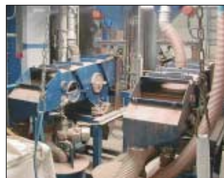
The upper fraction of inerts is separated from the broken particles and dust.
